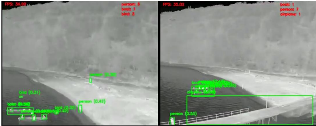
Fig. 1. Thermal camera images with analytical functions in coastal surveillance.
